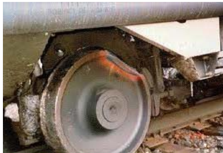
Fig.1 – Bandage wheel breaking.
